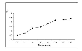
Figure 3 pH decrease during the treatment of olive mill waste waters with immobilized culture.
