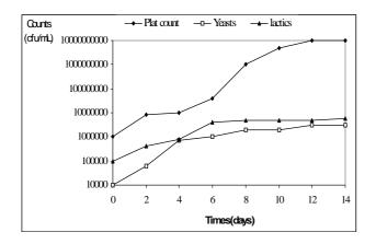
Figure 4 Microbial count profiles during the treatment of olive mill waste waters by the immobilized culture.
