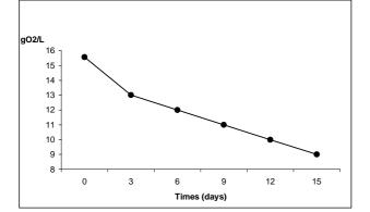
Figure 2 COD reduction by the immobilized culture in olive mill waste waters treatment assays.
