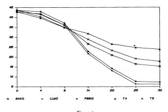
Figure 1 Time course (days) for the mean variations of the COD (g/l) TA = control type A waste water (inoculated with SNKD biological complex). TC= control type C waste water (inoculated with LLMO and PSBIO microbial formulations).
