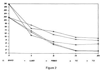
Time course (days) for the mean variations of the COD (g/l). TB= control type B waste water (inoculated with SNKD biological complex). TD= control type D waste water (inoculated with LLMO
