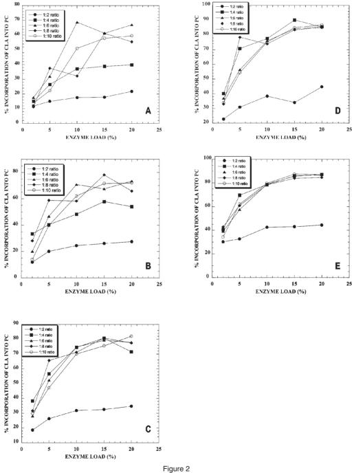
Effect of temperature on the production of SPC. A. 20 °C, B. 30 °C, C. 40 °C, D. 50 °C, E. 60 °C. Conditions: reaction for 24 h at 20, 30, 40, 50 and 60 °C; orbital shaker at 200 rpm; with 2, 5, 10, 15 and 20% enzyme loadings with respect to the weight of substrates.
