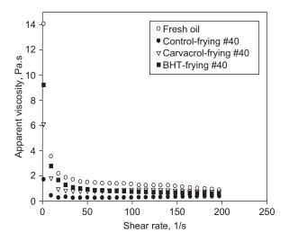
FIGURE 8. Changes in apparent viscosity as a function of shear rate for palm oil samples.
