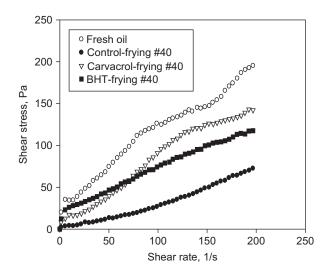
FIGURE 7. Changes in shear stress as a function of shear rate for palm oil samples.
