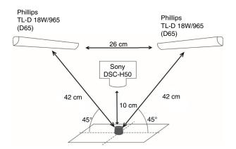
FIGURE 1. Digital image analysis set up.
