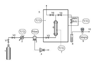
FIGURE 1. Supercritical carbon dioxide extraction apparatus. 1. CO<sub>2</sub> tank; 2. Cooling bath; 3. Pump; 4. Compressor; 5. Oven; 6. Extractor vessel; 7. Monitor; 8. Vial; 9. Flowmeter; 10. CO<sub>2</sub> Outlet; V1 – V6 Flow control valves; MMV Micrometric valve.
