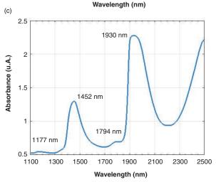
FIGURE 2. Examples of absorbance NIR spectra: a) fresh olive fruit; b) Arbequina extra virgin olive oil; c) water.
