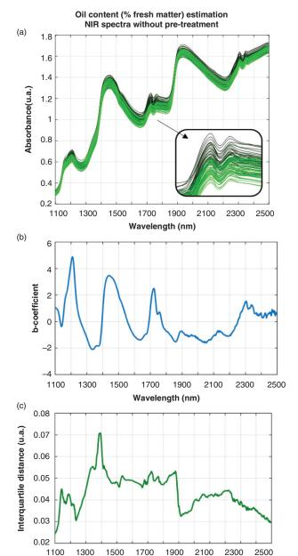
FIGURE 3. PLSR analysis for estimation of oil content (% fresh matter) from NIR spectra without pre-treatment: a) Absorbance NIR spectra of the calibration set; b) b-coefficients of the PLSR model with 6 latent variables; c) interquartile distance  $Q_{25-75}$ .
