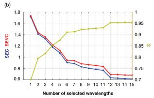
FIGURE 4. Procedure of variable selection for oil content (% fresh matter) according to the number of selected wavelengths introduced in the linear square regression model: a) Evolution of the explained variance X: NIR raw spectra matrix; Y: oil content (% fresh matter) matrix; b) Evolution of the standard error of prediction (SEP), standard error of cross-validation (SECV) and coefficient of determination (R<sup>2</sup>).
