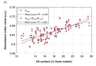
FIGURE 6. Oil content (% fresh matter) versus absorbance values (u.a.): a) The green series corresponds to index 1 values,  $I_1 = A_{1760}/A_{1724}$ ; b) The blue series corresponds to a raw absorbance value at 1724 nm ( $A_{1724}$ ); the red series corresponds to values computed as  $A_{1724}/(A_{1760}/A_{1724})$ ; b) The blue series corresponds to a raw absorbance value at 1206 nm ( $A_{1206}$ ); the red series corresponds to values computed as  $A_{1206}/(A_{1760}/A_{1724})$ .
