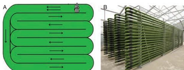
FIGURE 1. Surface view of a raceway ponds (A) and partial view of tubular photobioreactor (B) used for microalgae cultivation (Modified from Abomohra *et al.*, 2016).
