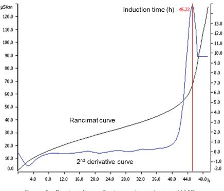
FIGURE 2. Rancimat diagram for *A. graveolens* seed extract (110 °C).
