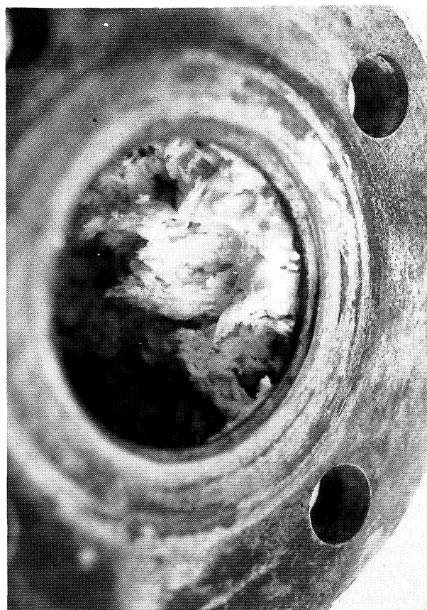
Figure 1 Stearic acid recovered in the neutralizing distillations, after the refrigeration system used to condense the distillates.
