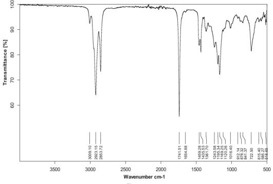
Figure 6 FTIR spectrum of maize oil methyl esters (MOMEs).
