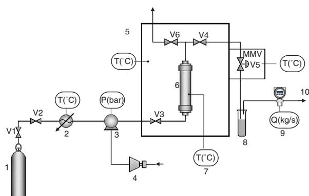
FIGURE 1. Supercritical carbon dioxide extraction apparatus. 1. CO<sub>2</sub> tank; 2. Cooling bath; 3. Pump; 4. Compressor; 5. Oven; 6. Extractor vessel; 7. Monitor; 8. Vial; 9. Flowmeter; 10. CO<sub>2</sub> Outlet; V1 – V6 Flow control valves; MMV Micrometric valve.
