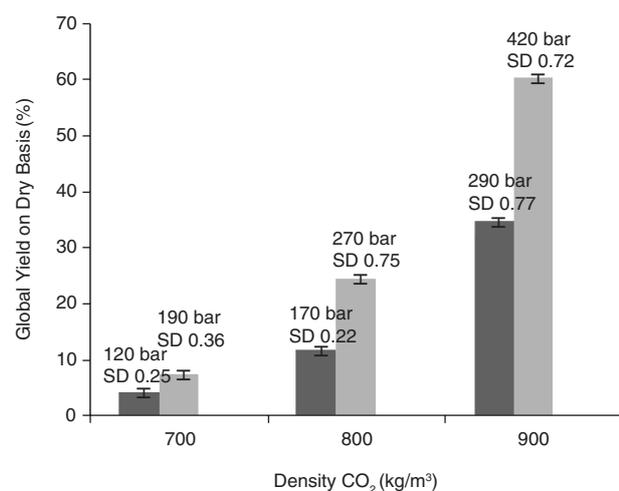
FIGURE 2. Supercritical CO<sub>2</sub> extraction isotherms yield on dry basis versus density of bacaba (*Oenocarpus bacaba*) oil. (■) 40 °C and (□) 60 °C isotherms. SD correspond to values of standard deviation of the yields.
