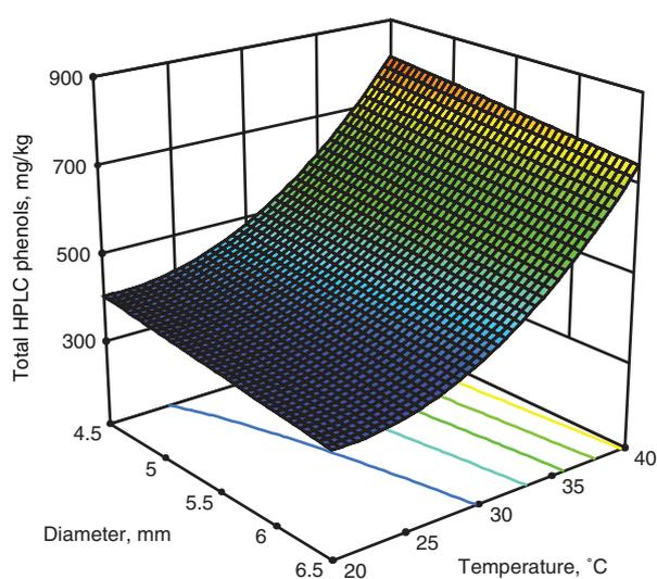
FIGURE 1. Effects of temperature and hole diameter of the hammer-crusher on total HPLC phenol content
