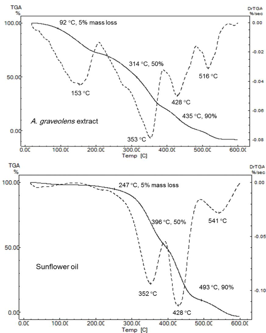
FIGURE 3. Thermogravimetric (TGA) and first derivative thermogravimetric (DTGA) curves of *A. graveolens* extract and sunflower seed oil.
