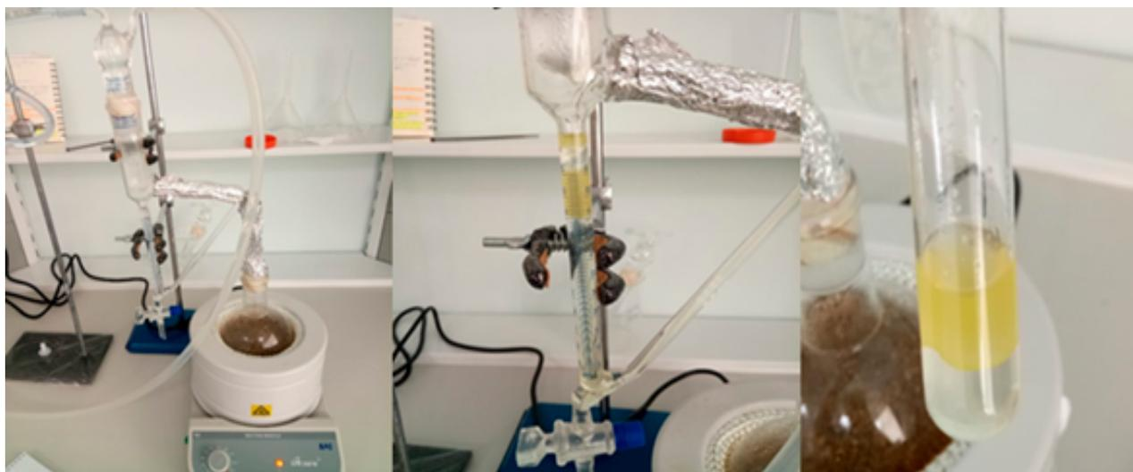
FIGURE 2. Essential oil extraction by Clevenger apparatus.
