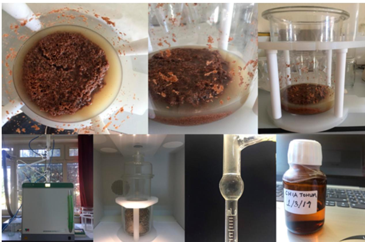
FIGURE 3. Essential oil extraction by microwave-assisted hydrodistillation.
