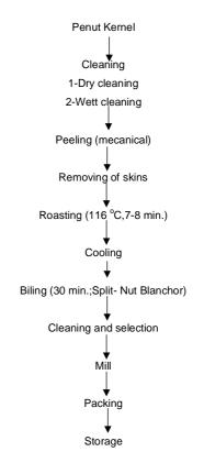
Figure 1 The Flow diagram of peanut butter production
