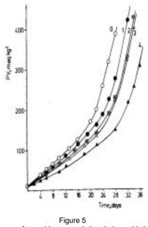
Kinetic curves of peroxide accumulation during oxidation of SO at room temperature under daylight at oxygen insufficient conditions (diffusion regime) in the presence of different  $\beta$ -carotene concentrations: 0 - 0%; 1 - 0.001% (1.86x10<sup>-5</sup>M); 2 - 0.005% (9.30x10<sup>-5</sup>M); 3 - 0.01% (1.86x10<sup>-4</sup>M); 4 - 0.02% (3.72x10<sup>-4</sup>M)
